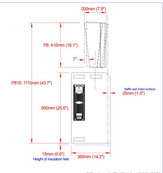
Baffle wall cut-out for P8 =  $480 \times 440 \text{mm} (19-3/4" \times 17-3/8")$ P815LF = 700 x 540mm (27-1/2" x 21-1/4") P815 = 1160 x 540mm (45-5/8" x 21-1/4") Weight P8 = 15.5kg (34.2Lbs) P815LF = 48kg (106Lbs)
